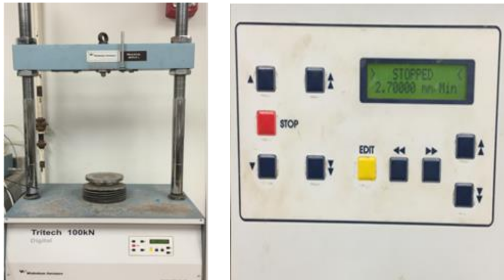
Figure 3. 11 Dynamic compaction machine
