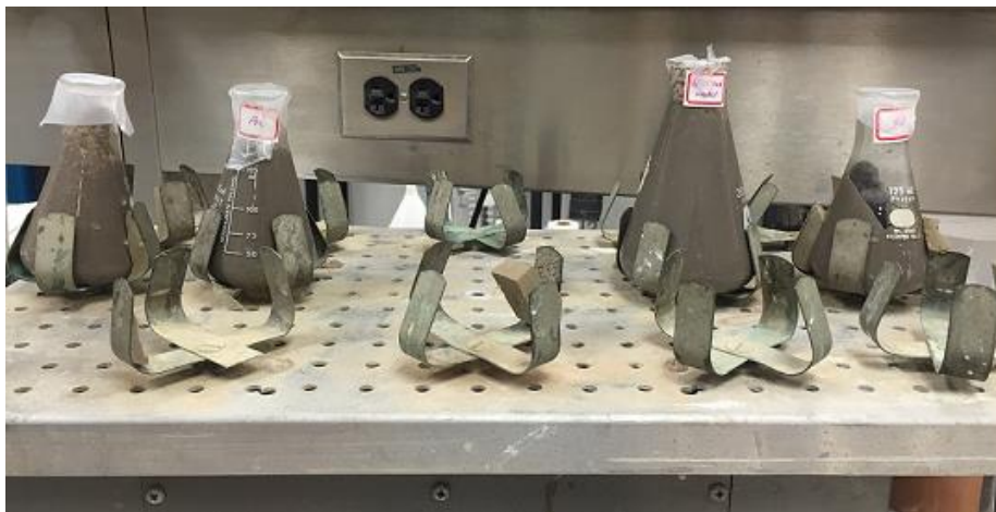
Figure 3. 19 Soil samples being shaken on shaking table
