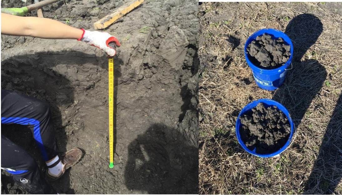
Figure 3. 2 Second soil sampling: 3 ft below ground surface
