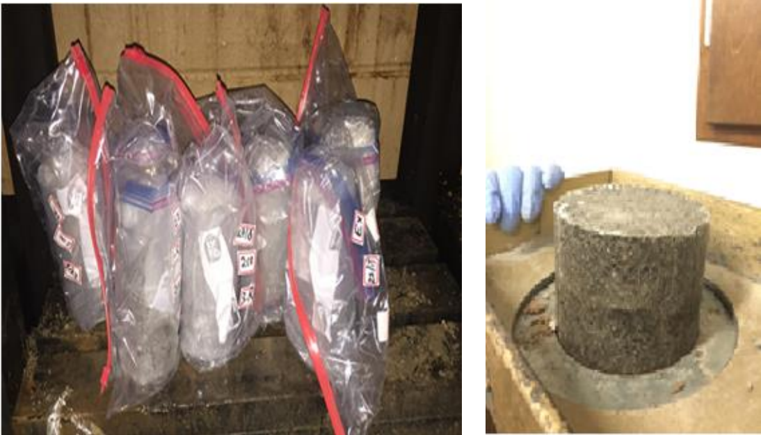
Figure 3. 12 Extruded and cured samples
